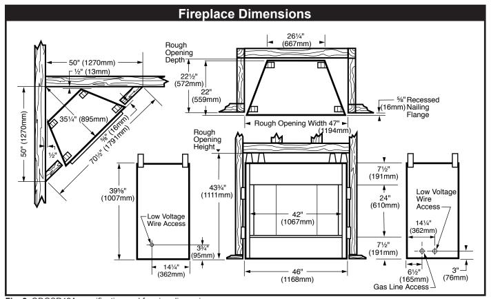
Fig. 2 ODGSR42A specification and framing dimensions.
