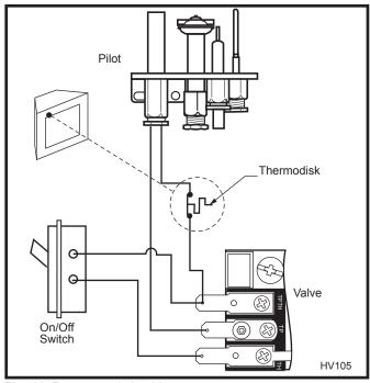
Fig. 11 Remote switch wiring.
