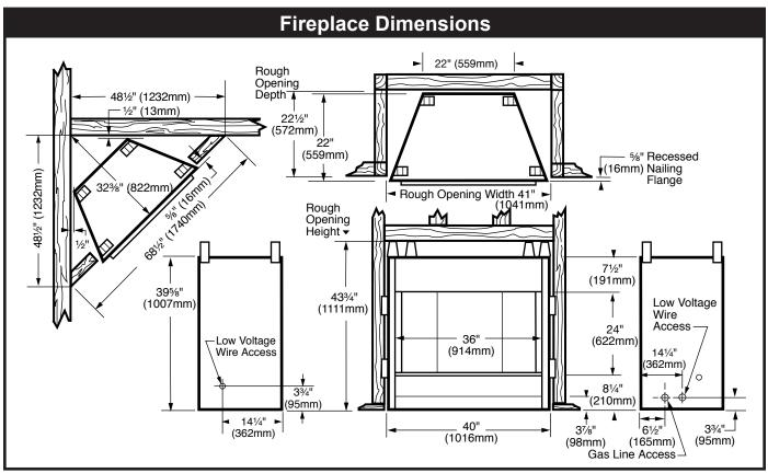
Fig. 1 ODGSR36A specification and framing dimensions.
