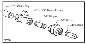
Fig. 10 Typical gas supply installation.
