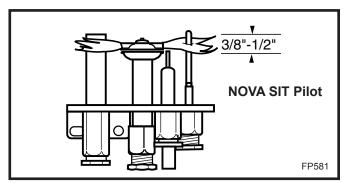
Fig. 16 Proper pilot flame height.
