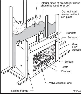
Fig. 9 Exterior chase installation.
