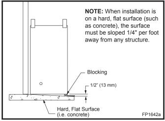
Fig. 7 Exterior chase installation.
