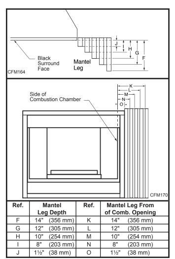
Fig. 3b Combustible mantel leg minimum installation.
