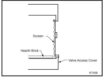
Fig. 20 Push bottom of weather enclosure into firebox.
