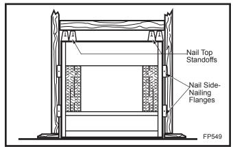
Fig. 4 Adjustable drywall strip (nailing flange).
