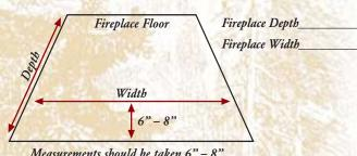
Measurements should be taken 6" - 8" inside firebox opening.
