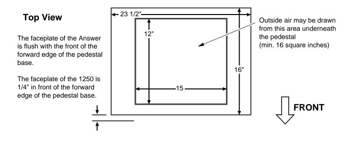
2 **Outside Air Cover Plate (<u>Required on the Answer ONLY</u>)** When using outside air with the Answer, install the cover plate to insure combustion air is drawn from below.
