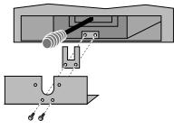
Attach the air control stop and cover plate as shown above. <u>HINT</u>: Place one screw through the cover plate and air control stop, and while holding them together, slide the components into place and tighten the screws to secure.
